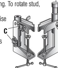
Tota-clamp has two snap-in fittings **C** for Flexi-shafts.
